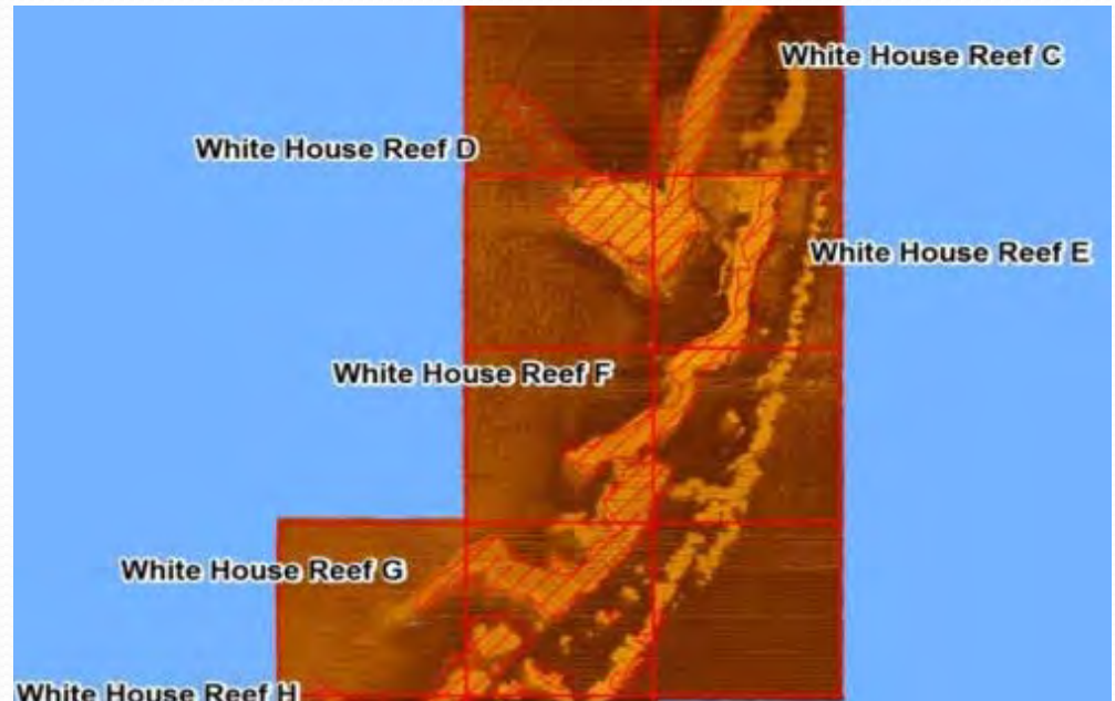
Mosaic of images obtained using side-scan sonar showing oyster reefs in Mobile Bay, AL
