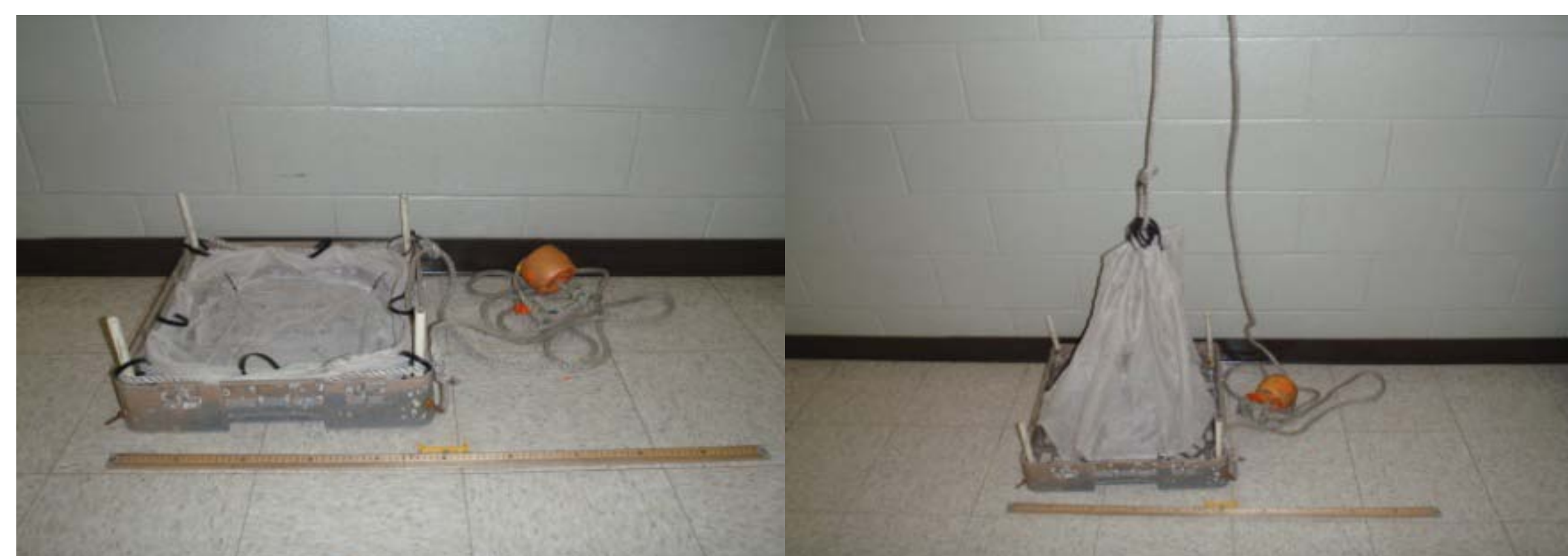
Figure 2: Modified sampling trays (0.22 m 2 ) used for this project were fitted with a collapsible drawstring mesh bag (1.6 mm) that enclosed the sample before retrieval.
