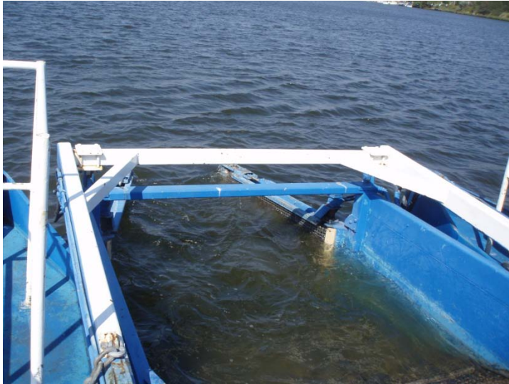
Intake conveyor ramp
